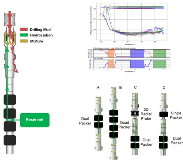
Figure 1: FTWT testing system shown with circulation unit and various inlet device configurations, together with an example pressure buildup dataset. Configuration options include A: Dual packer with two probes B: Quad-packer with two probes. C: 3D radial probe, probe and dual packer. D: Single and dual packer configurations.
