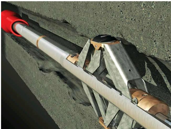
Figure 1: Formation tester in open hole
