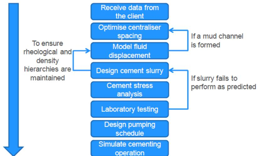
Figure 2: Typical design method for a cementing operation
