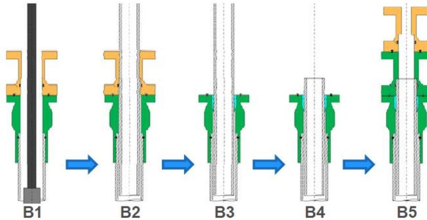
Figure 1: Simplified illustration of the installation process for a spool type wellhead
