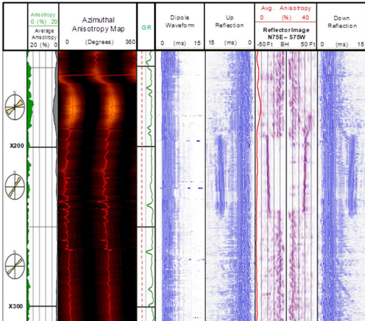
Figure 1 - Cross-dipole anisotropy results compared to the Deep Shear Wave Imaging looking out 50 ft from the borehole along the N75E-S75W azimuth; note the large vertical structure seen 30 ft away from the borehole over the interval from X195 to X240
