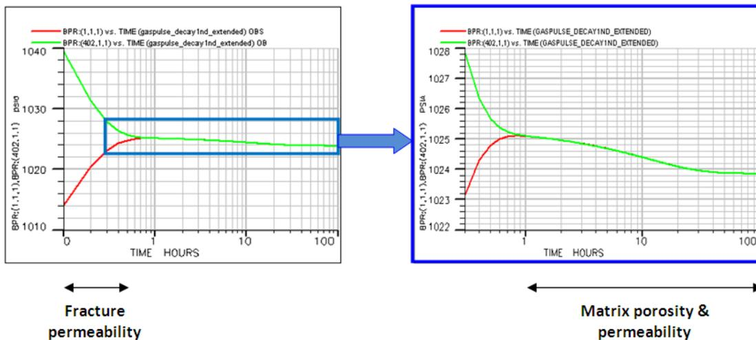
Figure 3. Simulation of an extended pulse-decay permeability showing fracture and matrix response. Gas permeability values lower than 0.001 nD ( $<10^{-24} \text{ m}^2$ ) are routinely reported from such tests. Those involved with seal analysis often use steady or unsteady state permeability analysis on core plugs using brine as the permeant. Published values obtained by such tests usually report
